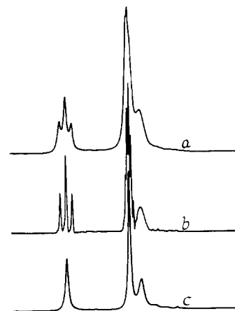
Figure 1. 86.7-MHz ^{11}B NMR spectra of neat (\mu-Me_2N)_2B_4H_8 : (a) normal; (b) line narrowed; (c) ^1H decoupled.
